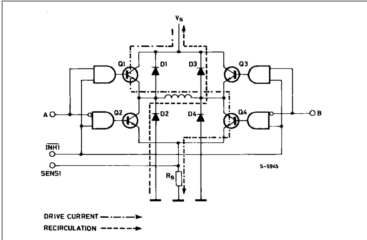
The L297 provides load current control in the form of two PWM choppers, one for each phase of a bipolar motor or one for each pair of windings for a unipolar motor. (In a unipolar motor the A and B windings are never energized together so they can share a chopper ; the same applies to C and D).
